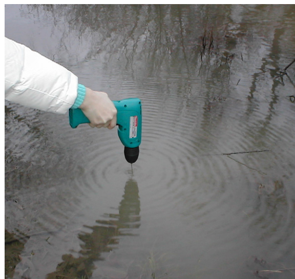
Fig. 4. On-site sampling of river water using the thin film sampler.
